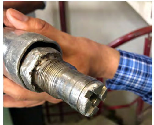
Damage to threads on SDX® III Nozzle.
